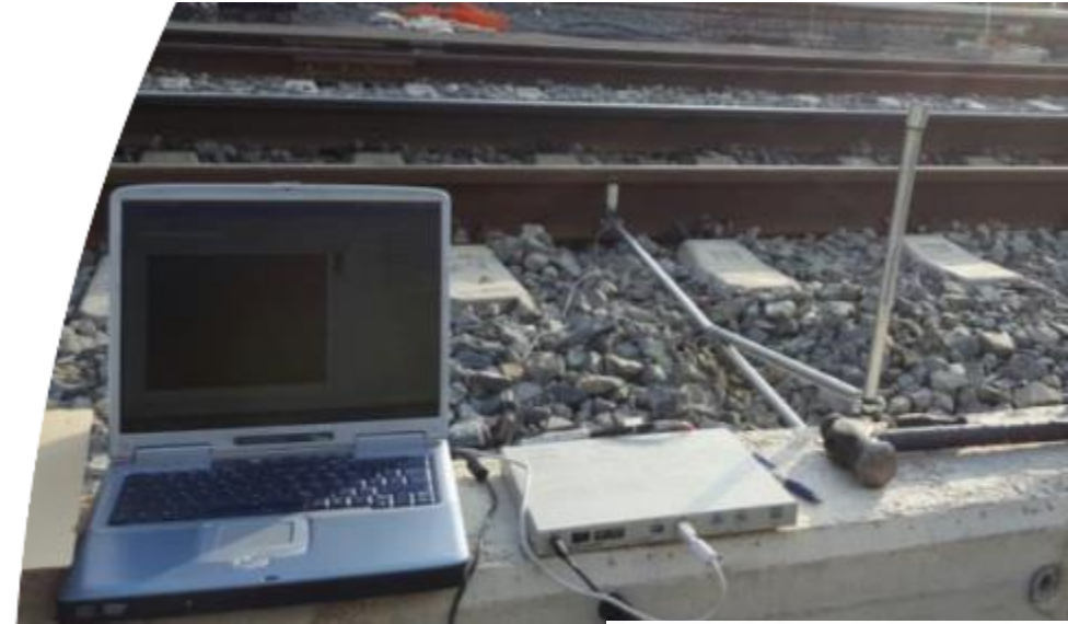
SSM/3G enabled, GPS device based on ATmega328 (Arduino)
